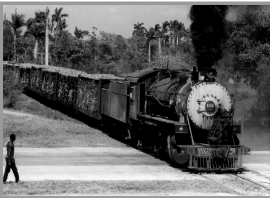
Trains Unlimited Tours 2002 excursion to Cuba featured many steam engines, mostly in use in sugar cane operations. This is the newest steam engine in Cuba- a 1935 built Baldwin Mikado (2-8-2) in one of three photo crossings of one of Cuba's few rural 4 lane highways. Photo by Wallace
